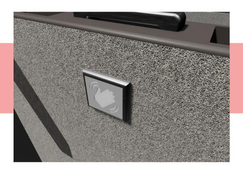
The hand sensors allow the customer to swipe their hand over them and instantly have the panels open up automatically for them. The sensors would only detect the swipe of a hand and not a foreign object to avoid having them open in the trunk randomly.
